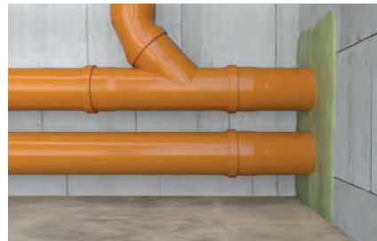
Filling pipe penetrations
