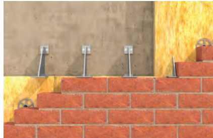
Insulating materials in two-leaf external walls
