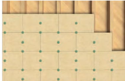
Flush mounting of mineral wool boards
