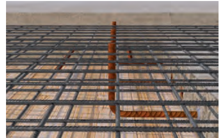
Post-installed rebar connections
