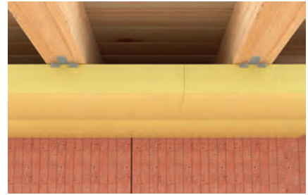
Pressure-resistant insulation boards on ceiling undersides
