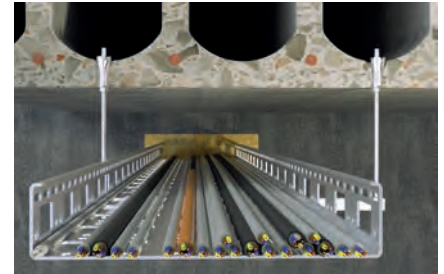
Cable trays in pre-stressed hollow-core concrete
