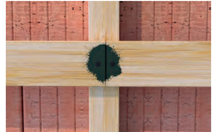
Sealing of the screw heads
