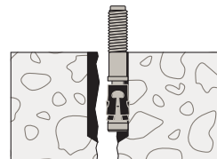
Concrete splitting failure
