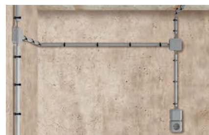
Flexible and rigid plastic pipes
